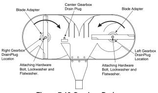
Figure 7-13 Gearbox Drain
